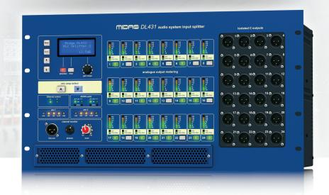
DL431 is a 6U 19" fixed-configuration rack I/O unit designed for microphone signal splitting applications with 24 mic/line level inputs and 72 line level outputs, and delivers legendary MIDAS sound quality utilising our time-tested and road-proven technologies. Featuring two independent MIDAS microphone preamplifiers with 2.5 dB gain steps plus a third fixed gain MIDAS
