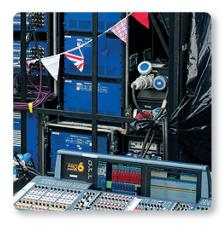
Microphone preamplifier per input channel, two dual redundant AES50 network interfaces, dual redundant Ethernet control ports and a MIDI Interface (In, Out, Thru), the DL431 is the ideal partner to the MIDAS PRO3, PRO6, PRO9, XL8 and PRO X digital consoles, enabling a digital snake connection from Front of House to stage.
